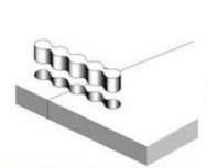
Metalock keys are driven into the openings and caulked.
