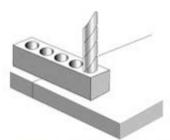
Using a drill jig, rows of blind holes are drilled perpendicular to the direction of the crack, each row to act as a key.
