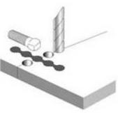
4. Holes for Metalock screws are drilled along the crack between the keys.
